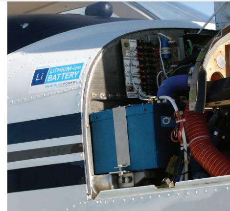
Installation of TB17 Certified Lithium-ion Battery in A36 Series Bonanza
