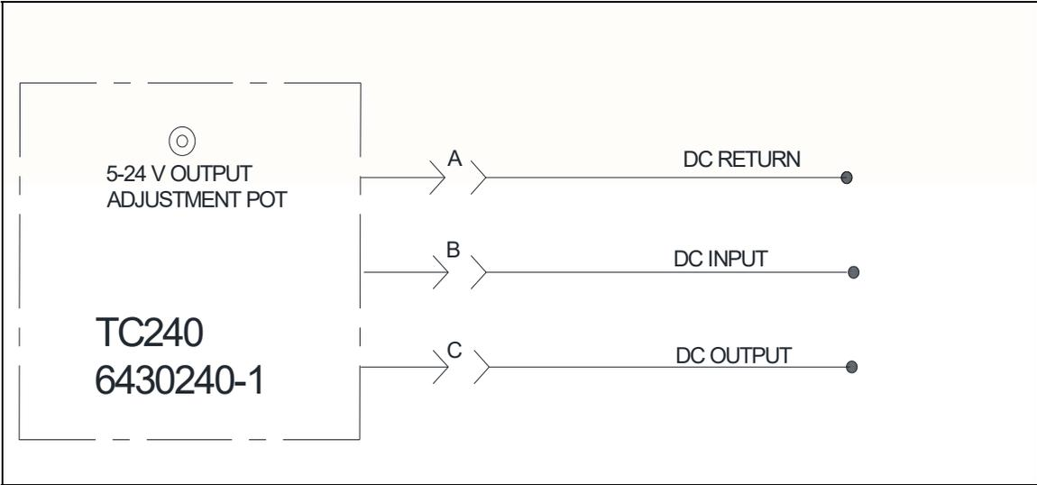
**Figure 3.3: Typical 6430240-1 Aircraft Wiring Installation – Constant On**
