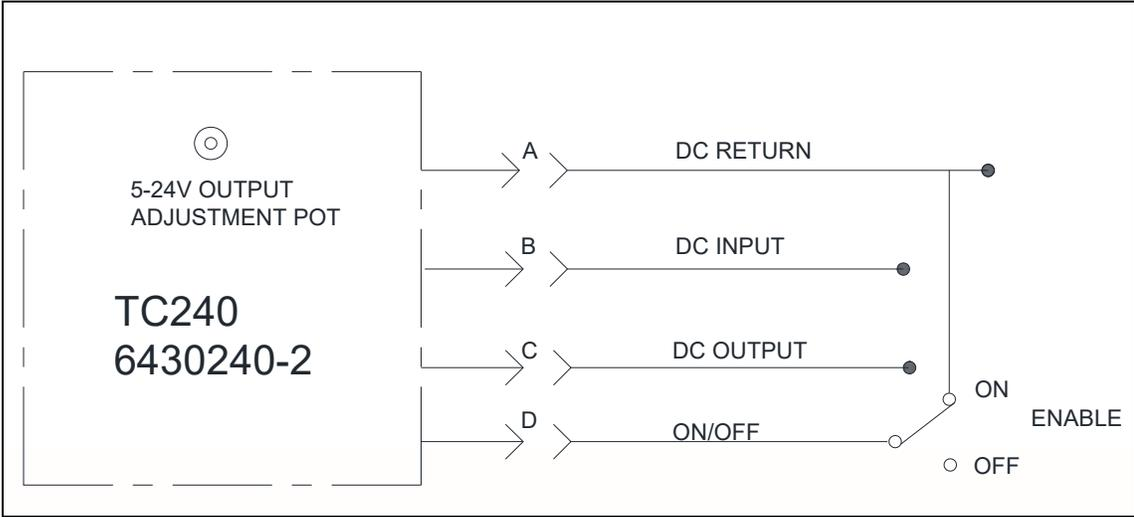
**Figure 3.4: Typical 6430240-2 Aircraft Wiring Installation – Remote On/Off**
